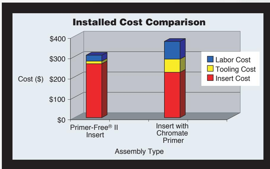
The chart above illustrates the significant difference in installed cost when comparing Primer-Free® II inserts with inserts coated with liquid chromate primer. Significant savings - in excess of 20% - can be achieved when utilizing Primer-Free® II inserts. These savings are largely due to the elimination of the application of the liquid chromate primer, which is a labor intensive process and often results in inconsistent coverage of the threads.
