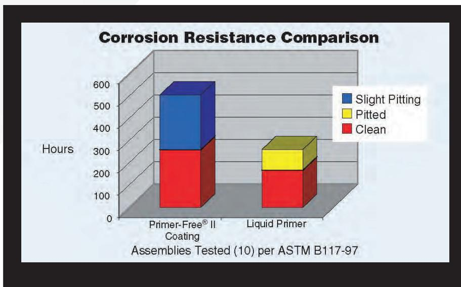
Primer-Free® II inserts have undergone extensive salt fog testing per ASTM B-117. After exposure, the samples were sectioned to expose the threaded insert for examination. When protecting against galvanic corrosion, Primer-Free® II inserts did consistently meet or exceed the performance of insert assemblies containing liquid chromate primer.
